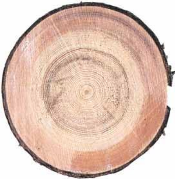
The disc contains aniline wood, which marks the tree's defence zone against root rot attack. The wood is not rot damaged in this stage.
