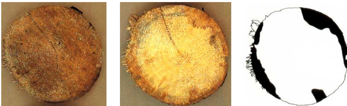
Figure 7. Storage decay in spruce. Left: end surface of the log; Middle: a cross-section 15 cm from the log end; Right: Storage decay highlighted in black. Log diameter 20 cm, 25% storage rot (Rötskador i massaved, Swedish Forest Agency, 1989).
