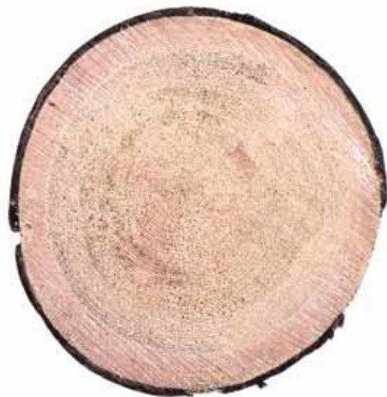
In this disc, light, solid rot has formed inside a weakly coloured zone of aniline wood. Light, solid rot is not counted.
