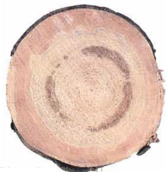
Disc with patches of dark, solid rot. Only these are counted. Slightly developed aniline wood.
