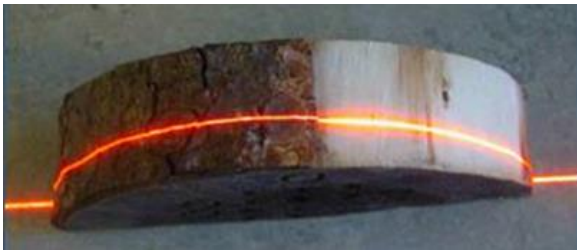
Figure 8. Principle of diameter measurement under bark using the tracheid method The laser beam used in the scanner is more dispersed on wood than on bark. Image analysis measures the width and intensity of the laser beam, distinguishing between wood and bark.
