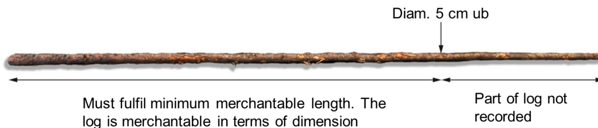
Figure 1. For logs with diameters of 50 mm at minimum length, but less than 50 mm at the top, the part where the diameter is less than 50 mm is not recorded.
